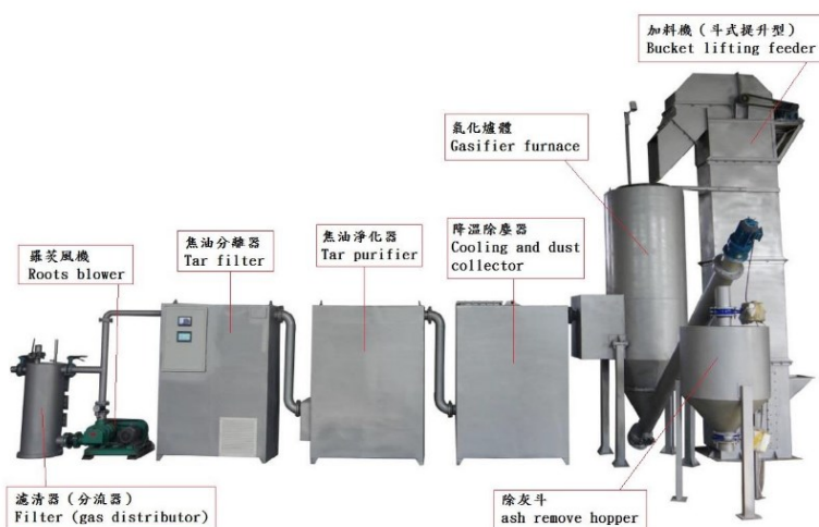
Figure 2. 100KW biomass gas power generation equipment
